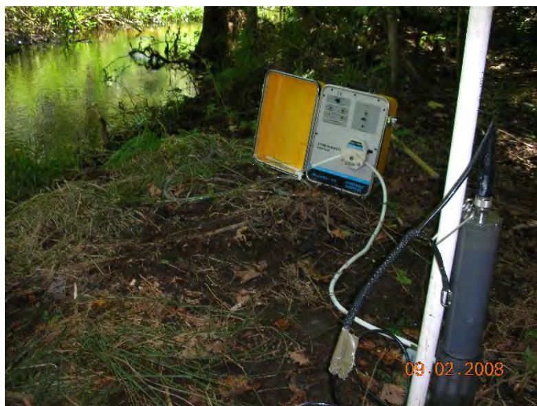
Picture 3. In-situ Measurement of Pore Water Properties.
