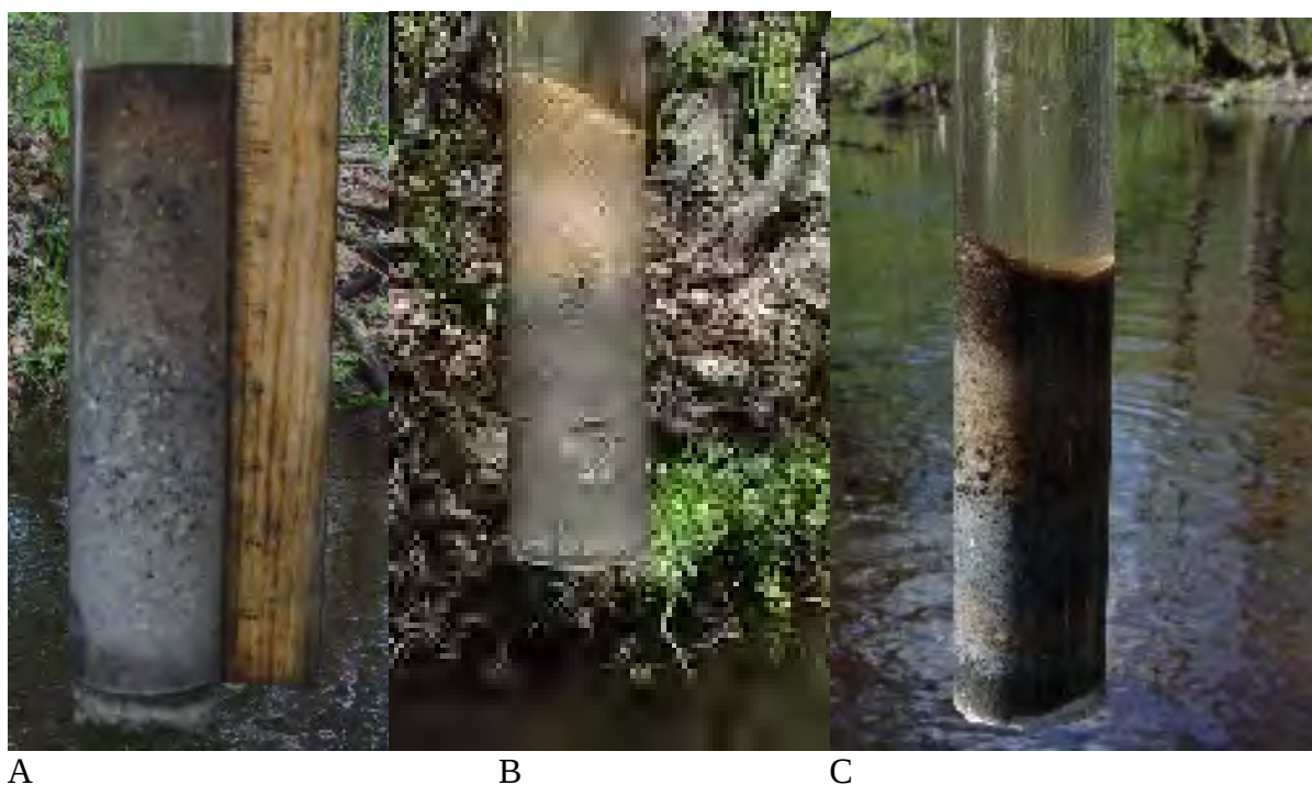
Picture 24. Sediment Cores Collected from Depositional Areas after Six Months - biopolymer/apatite/organoclay/sand cap (A), apatite/sand cap (B), and biopolymer/apatite/sand cap (C).
