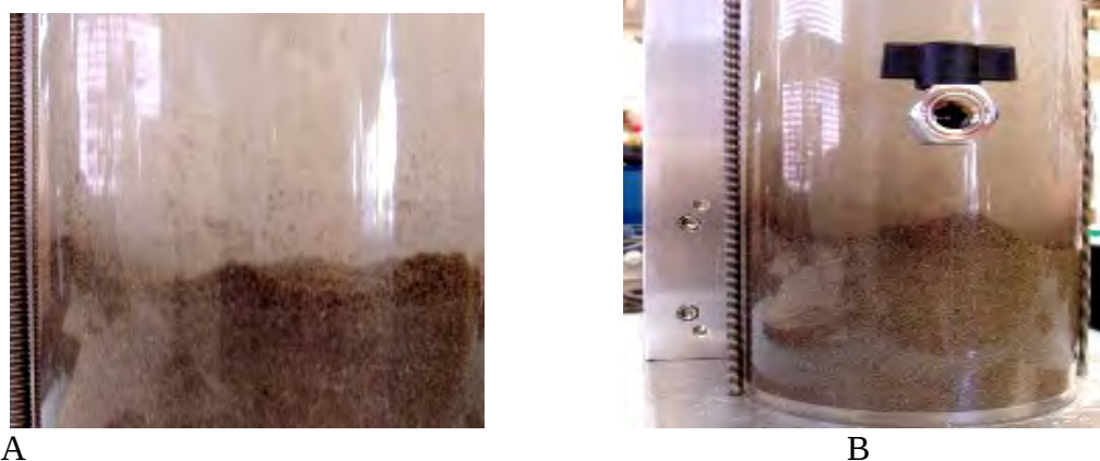
Figure 78. Resuspension of Organoclay (PM-199) leading to Cloudiness (A) and Surface Suspension (B).
