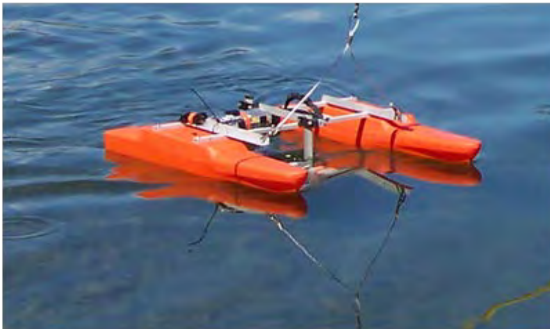
Figure 4. Surface mini-catamaran with downward-looking ADCP.
