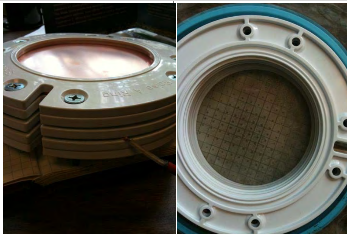
Figure BII-2. Pictures of the Micromegas detector prototype assembled in the Department of Physics at the University of Pennsylvania. Left: the gray rings seal the electrodes and micromesh with O-rings. Gap spacings can be changed by mounting the electrodes and/or the mesh in different slots in the gray mounting rings. A wire for one of the high-voltage electrodes is visible. Right: with one of the electrodes removed, the micromesh is visible inside the chamber.
