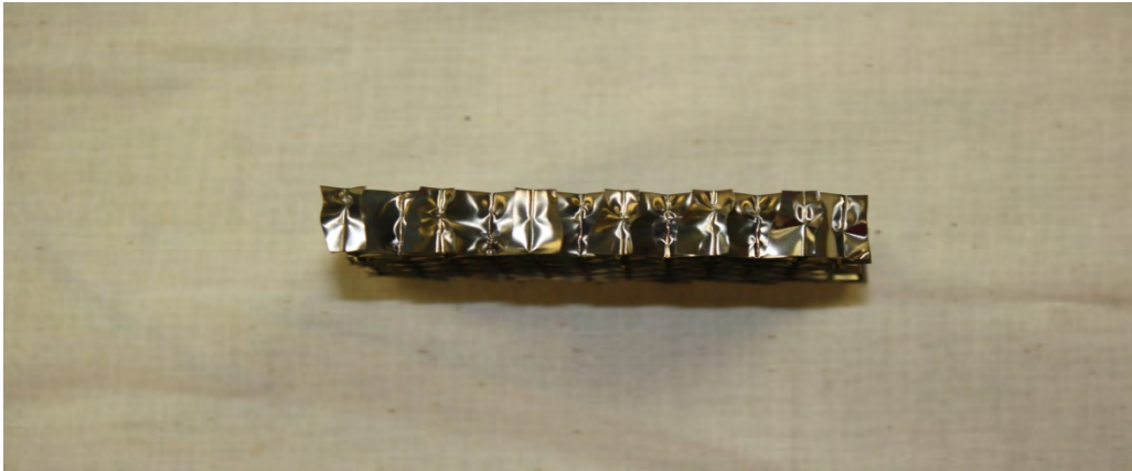
Figure 1: Uncoated Titanium Honeycomb Core after Compression Test
