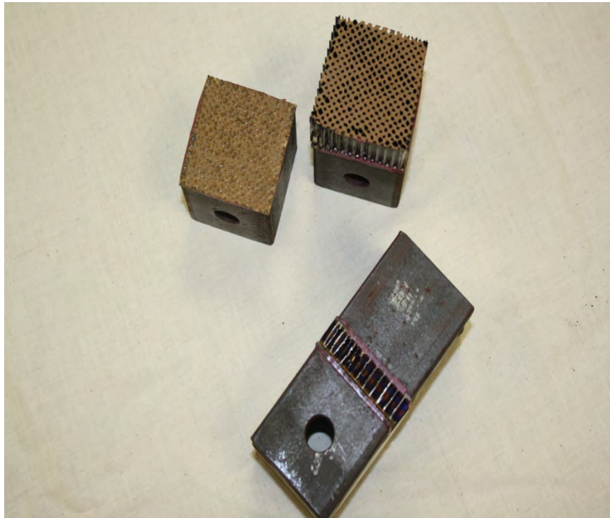
Figure 5: Tensile Test Specimens Pre- and Post- Testing
