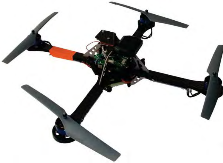
Figure 1. AscTec Hummingbird Quadrotor (After [1])
