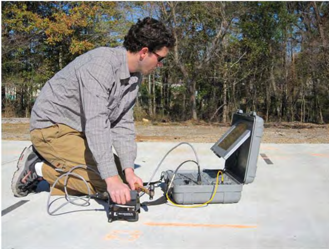
Figure 21. Impact echo testing.
