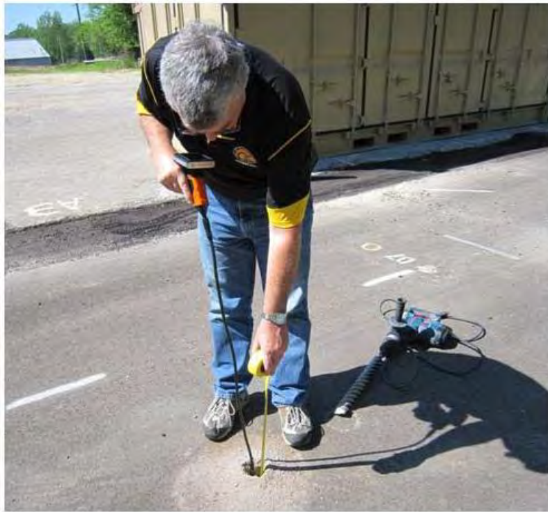
Figure 40. Using the borescope and measuring tape inside the drilled hole.
