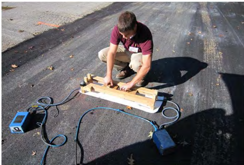
Figure 25. Common midpoint testing using two 1.5-GHz GSSI antennas.
