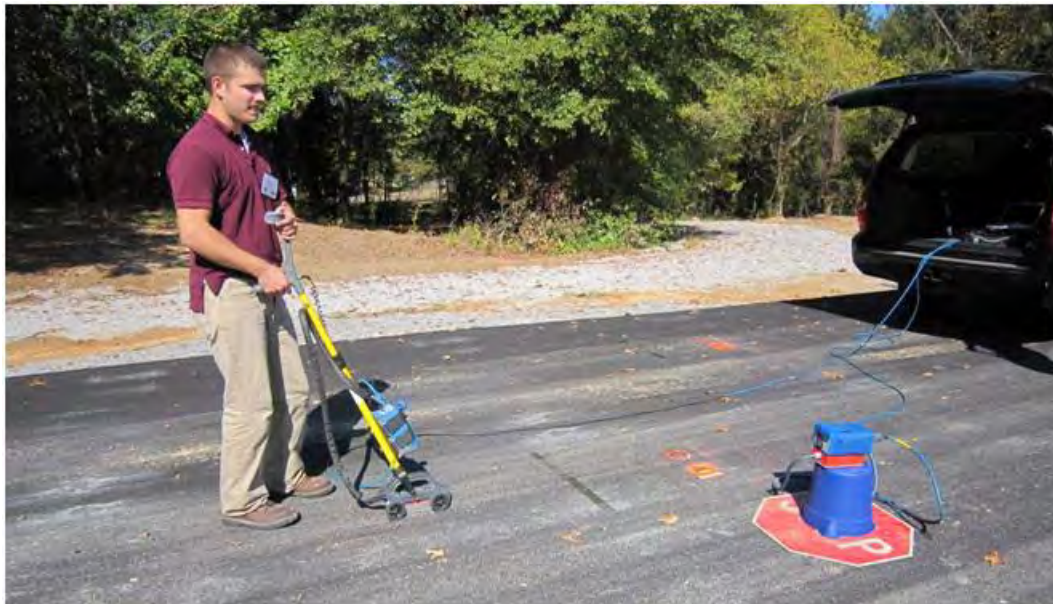
Figure 23. Single 1.5-GHz ground-coupled GPR testing.
