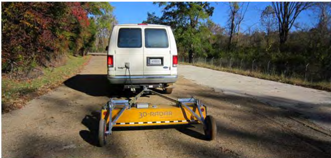
Figure 36. Testing with the 3D-Radar system.
