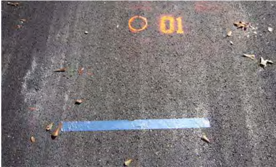
Figure 16. Test location marked with a circle to indicate location of the core hole and metallic tape spaced 2 ft away from the center of the core hole.
