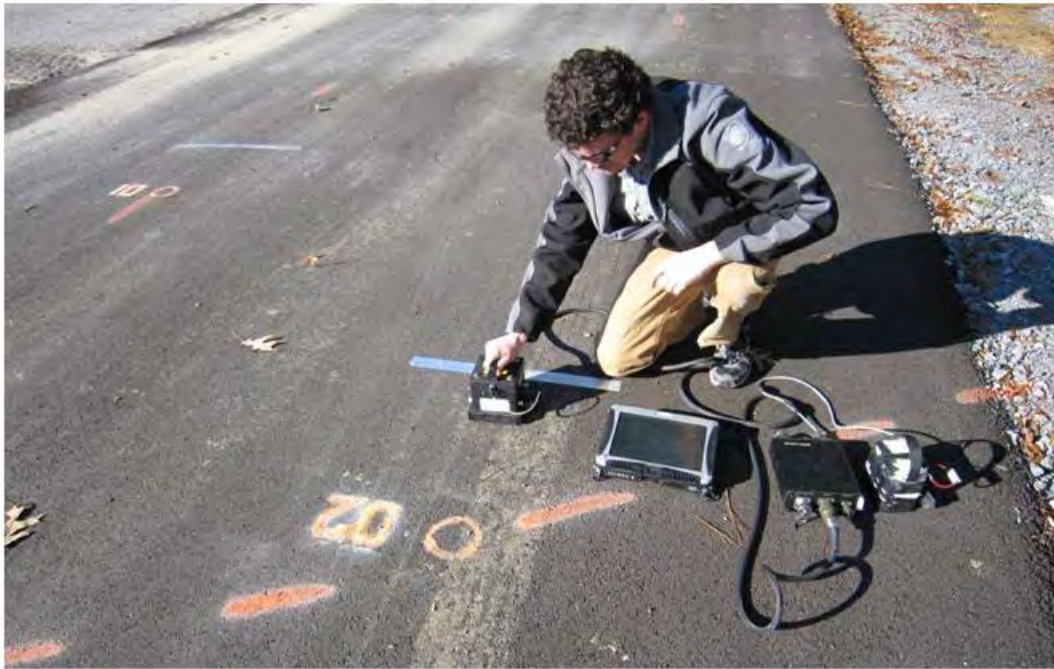
Figure 22. 2-GHz Ground-Coupled IDS Aladdin GPR (Olson Engineering) testing.
