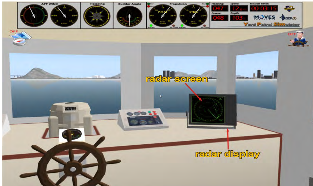
Figure 40. YPSim's radar screen displayed on the radar unit, inside the bridge.
