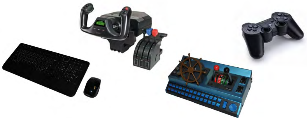
Figure 19. YPSim input devices. From left to right: keyboard/mouse, flight yoke, Ship Driver Controller(TM), and PS3 controller.
