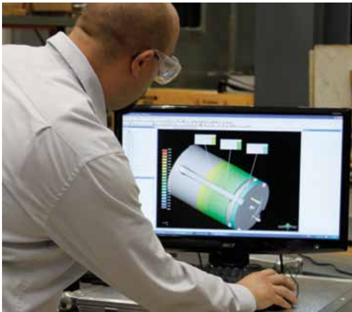
NMC is developing a white light scanning system for inspecting tapers of main propulsion shafts. The project is expected to save ship construction and maintenance costs. NMC photo
