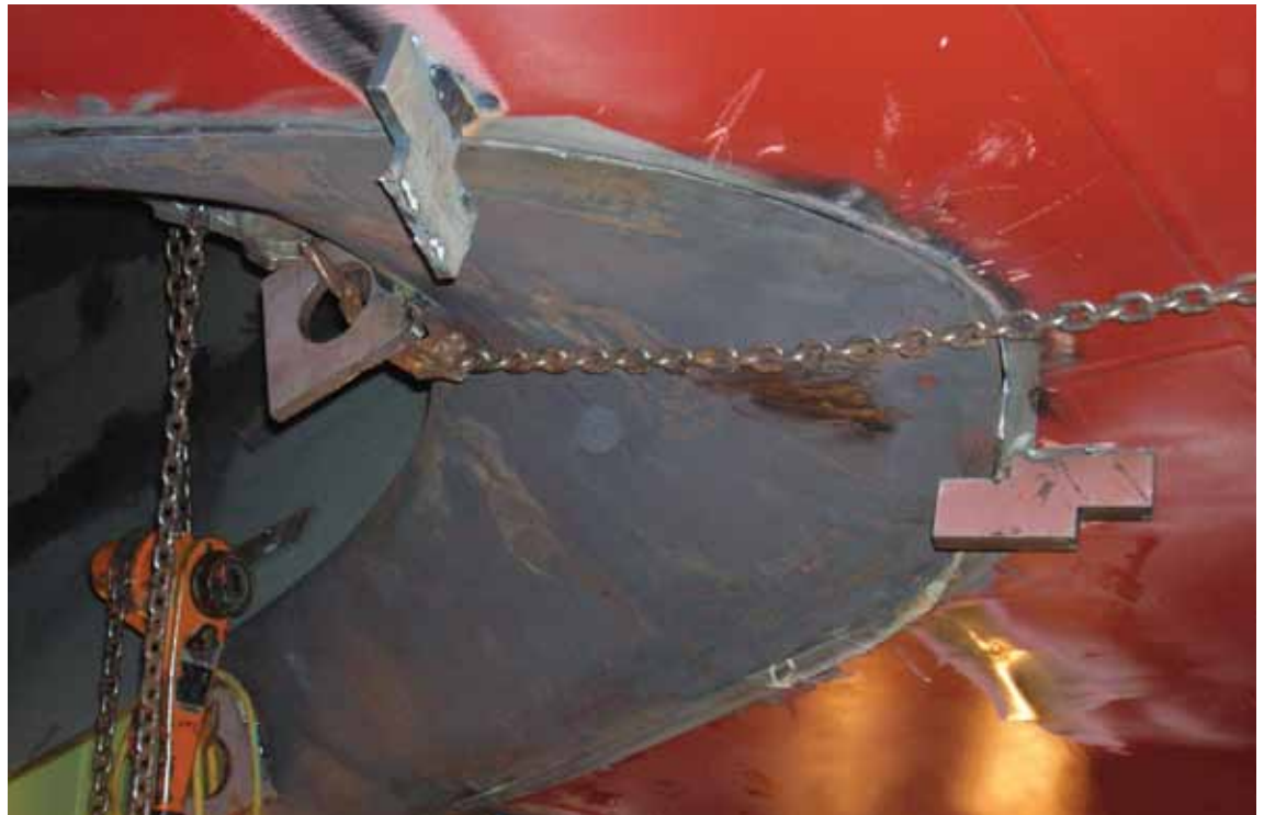
An NMC project used advanced techniques to design and manufacture the casting mold for the Freedom-class LCS waterjet entry edge. The cast component will save significant labor hours, improving the shipyard's ability to produce multiple ships. MMC photo
