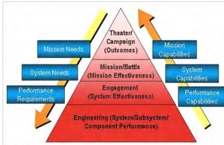
Figure 1. Relationships between the various types of system models and their effect on the overall outcome (From Standard, 2010)
