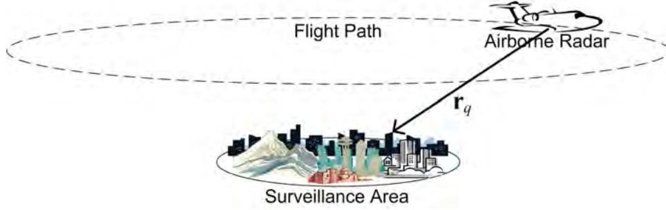
Figure 6. Vector from the antenna phase center to the q th scattering center.
