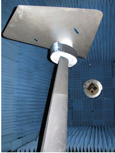
Figure 31. Photo of D2 airframe from a rear aspect [4]. The D2 is on the target pedestal at the AFIT Indoor RCS measurement range with the radar antennas shown in the background.
