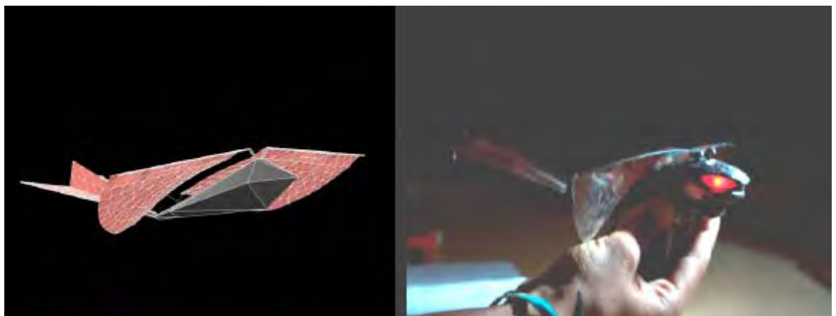
First dominant vibration mode for the MAV toy and the computational model.
