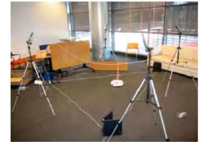
Experimental set-up: four cameras in a well-lit conference room. The entire system is controlled by a laptop computer on the table in the background.
