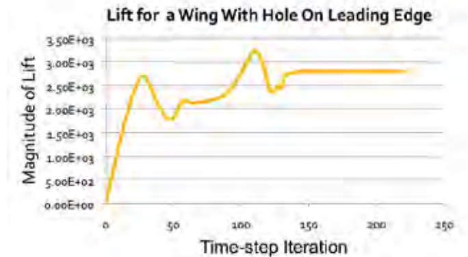
Simulated lift for a wing with a hole in the leading edge. With every iterative segment, the solution became more accurate, reaching a steady state oscillation around the correct value.
