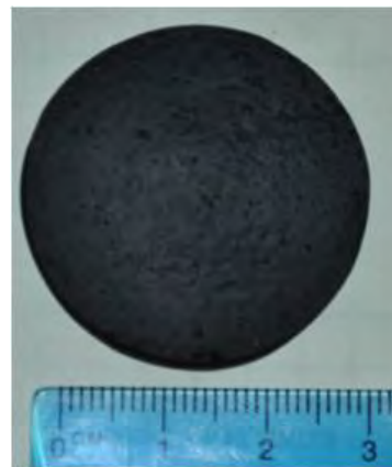
Figure 3.1-2: Photograph of multi-layer substrate with 200 mg of 20-40 nm \text{Fe}_2\text{O}_3 nanoparticles in the middle layer at a filtration pressure of 20 psi.
