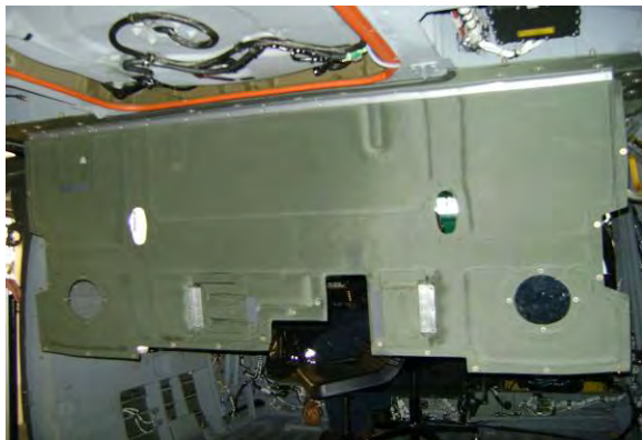
Sample 332 – Ceiling Panel Assembly
