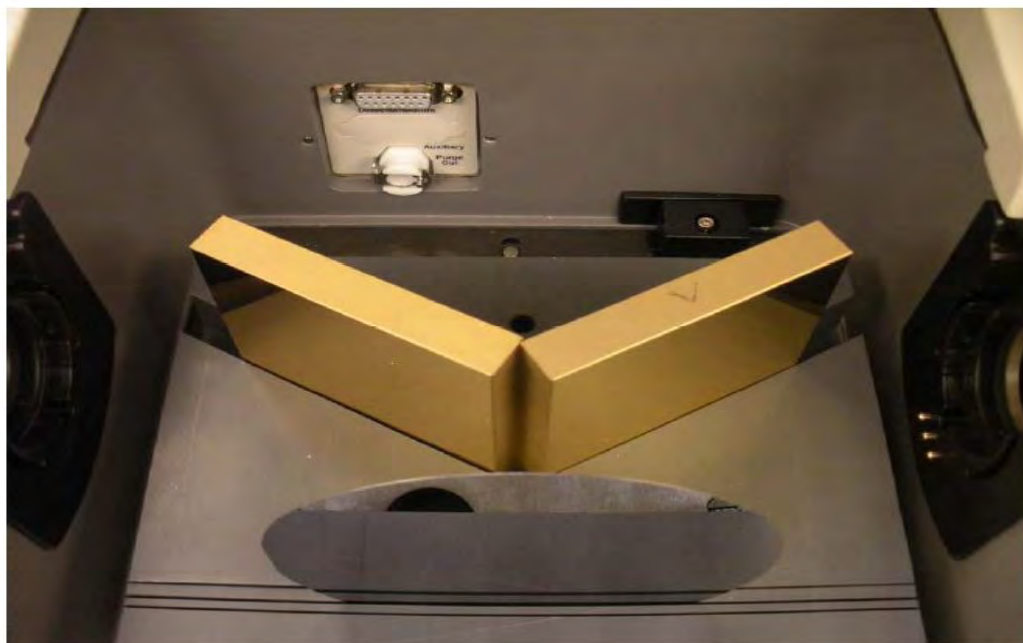
Figure 12. Sample compartment of FTIR showing the placement of the sample in the reflection measurement.
