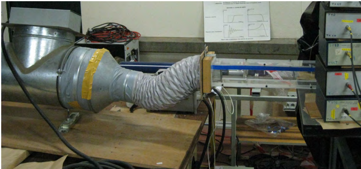
Figure 28: Upstream Heat Exchanger
