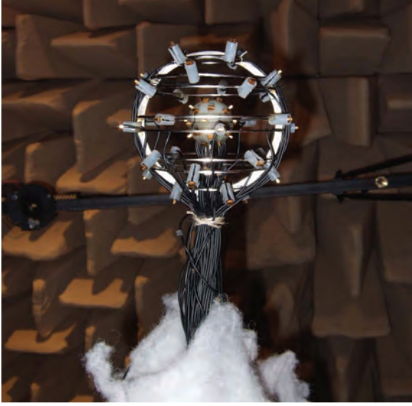
Fig. 1. A photo is showing the dual, concentric SMA located inside the anechoic chamber in which its' performance was measured. The moveable loudspeaker is shown to the left of the SMA.
