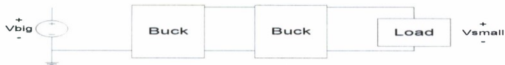
Figure 20. Conventional method to step down battery voltage
