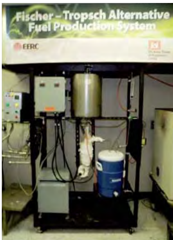
Figure 31. Small-scale FT reactor system for testing small quantities of catalyst with synthetic syngas.
