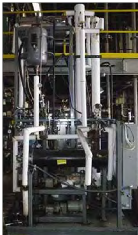
Figure 32. Large-scale FT reactor for testing large batches of catalyst with coal- or biomass-derived syngas.
