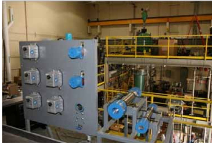
Figure 5. Monolith pressure vessels and valves and regulators that control gas flow during adsorption and desorption testing. The open pilot plant setting can be seen behind the test system.
