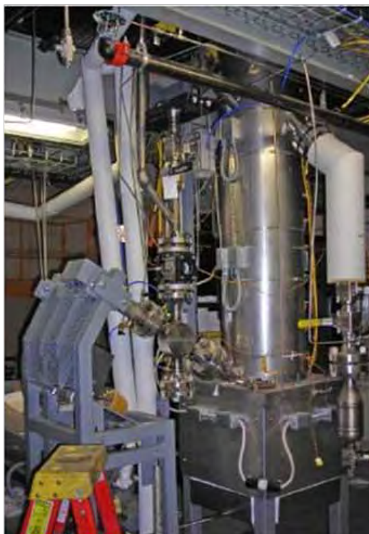
Figure 34. Photograph of the lower section of high-pressure fluid-bed gasifier. Visible at left is the feed auger angled downward into the bed.
