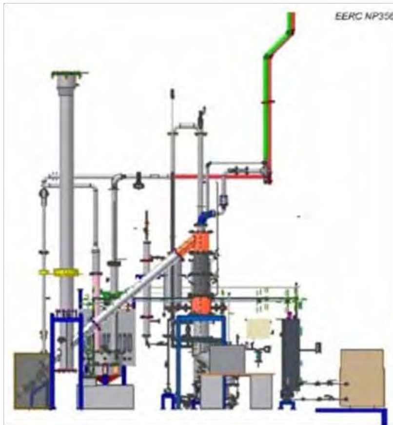
Figure 17. Three-dimensional view of the pilot plant gasifier depicting the major components of the system.
