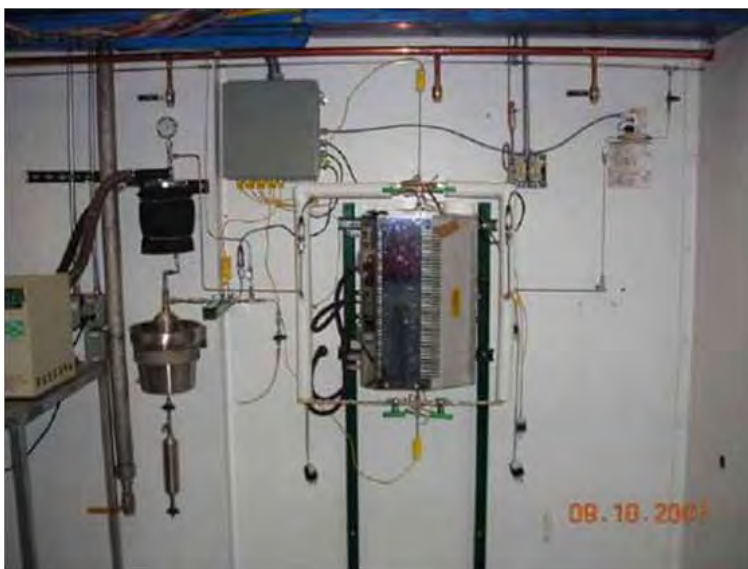
Figure 51. Small continuous reactor system used for kinetic rate data experiment.
