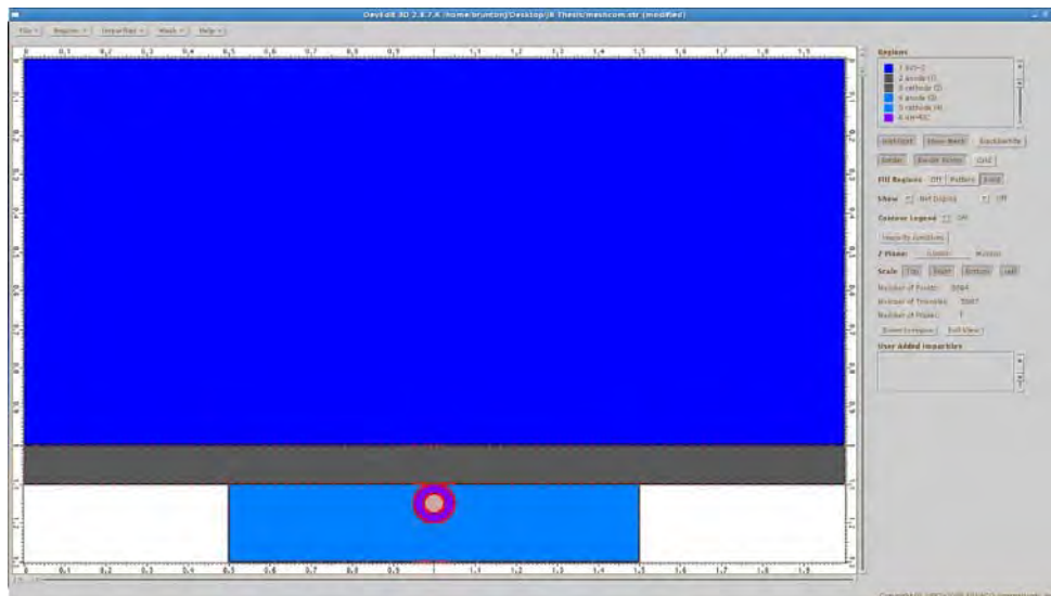
Figure 17. Cross-section of 3D device with circular CNF.
