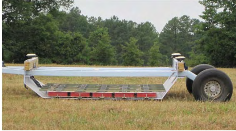
Figure 2-6 – Sensor array mounted on the MTADS EMI sensor platform.
