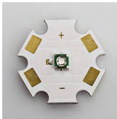
Figure 12. Cree XLamp XP-E LED Green: used as the visible light source for the readout. From [43]
