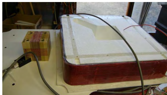
Figure 2-2 – Individual updated TEMTADS EMI sensor with 3-axis receiver under construction.
