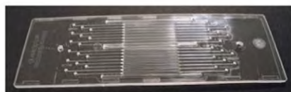
Figure 1. Microfluidic thermal cycling for PCR and Sanger sequencing. A) Rapid, Peltier-based thermal cycler; B) 16 sample microfluidic biochip (dimension 25×75 mm). doi:10.1371/journal.pone.0010595.g001
