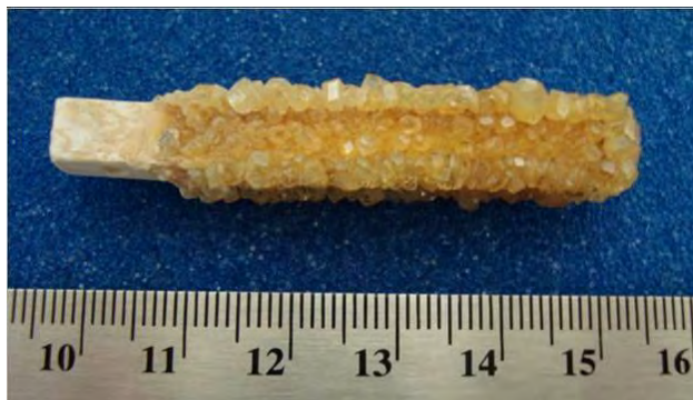
Figure 20. Photo of a ceramic rod from Konoshima after an attempt at liquid phase epitaxy.
