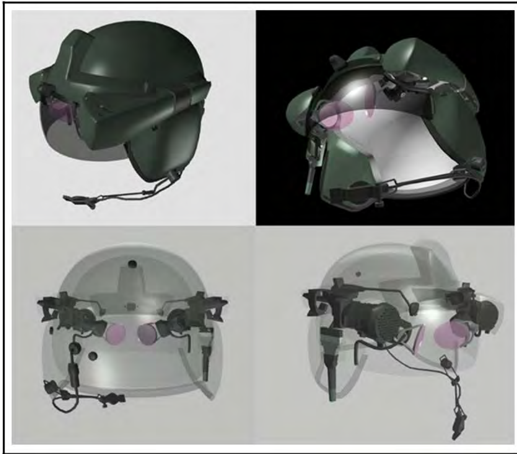
Figure 12. 3-D rendering of the HIDSS.
