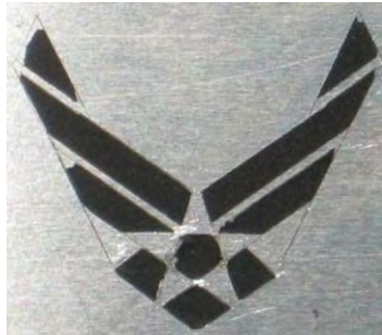
Fig. 4. USAF symbol target composed of absorptive tape on brushed aluminum.
