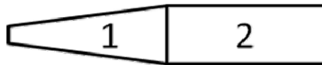
Fig. 1. Non-symmetric sensing strip design capable of acting as a 2×1 sensor, with regions 1 and 2 denoting different force sensing areas.
