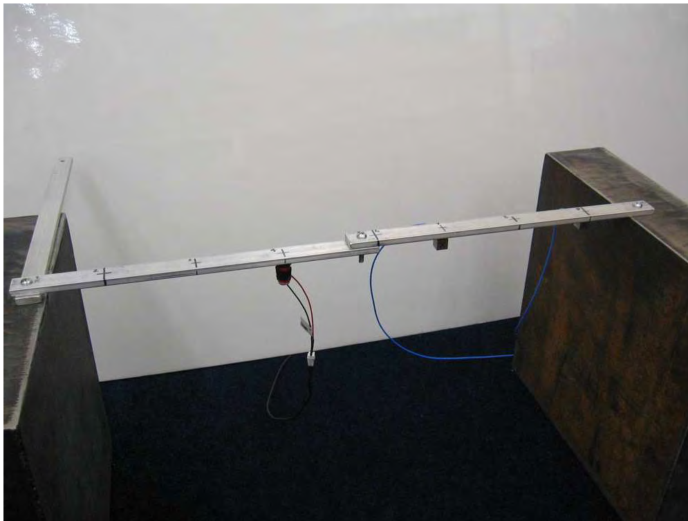
Figure 5: Two-beam, one-bolt setup with fixed boundary conditions.
