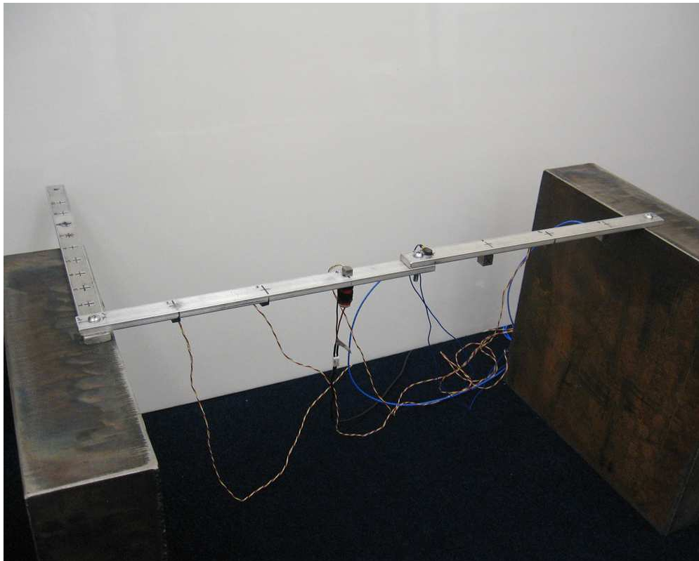
Figure 12: Two-beam, one-bolt setup with sensor array.
