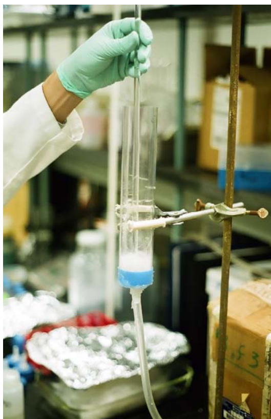
Figure 14. Packing leaching column with a base of glass wool to retain solids.
