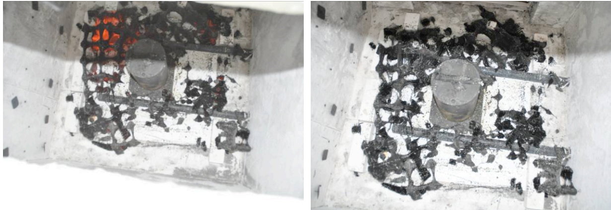
Figure 15. Test 6 photographs of the late-test burnout. The left photograph shows minor glowing in several regions of the collapsed crib. The right photograph shows a similar view at a later time. Air enters from the top of these photographs.
