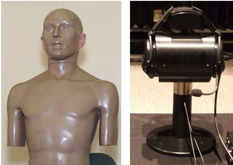
Figure 2. Auditory test fixtures used for measurement of the candidate systems: (left) KEMAR acoustic manikin § and (right) G.R.A.S. Hearing Protector Test Fixture Type 45CA (shown with TEA circumaural headset).
