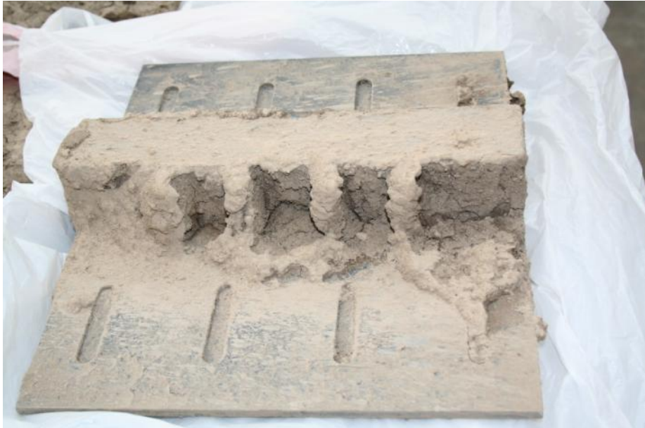
Figure 5. Soil and seed mixture on seed loss plates after being driven a specified distance on a wet road.
