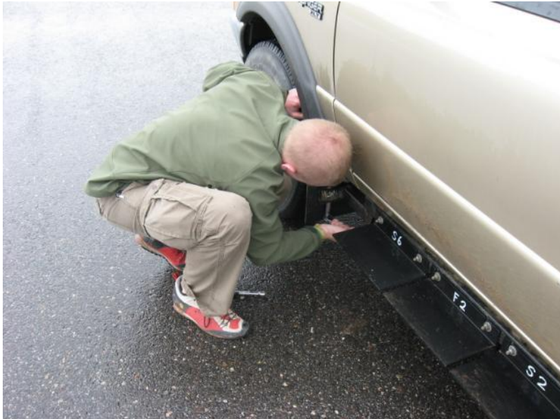
Figure 4. A wheel well plate being attached to the retention frame of a 4x4 wheel drive truck to which underside plates have already been bolted.
