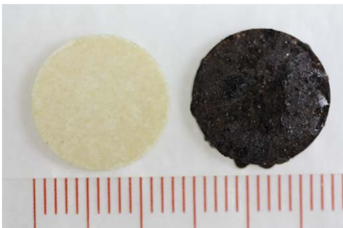
Figure 24. One Comp-B preparation was amended with unencapsulated, powdered NaOH (right disk), but proved too reactive during casting for self-remediation testing.
