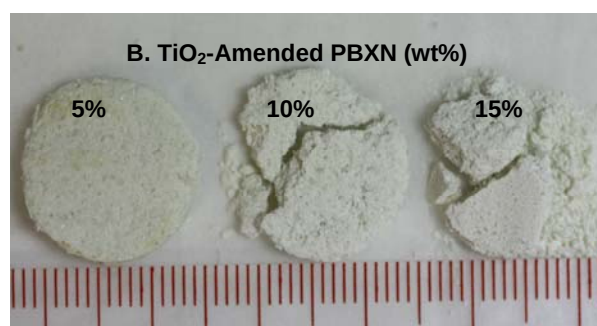
Figure 2. Photographs of PBXN-107 preparations: (A) unamended; (B) \text{TiO}_2 -amended; (C) Fe-amended, and (D) FeNi-amended. Note heterogeneity in all samples and the friable nature in all amended samples except the 5%- \text{TiO}_2 .
