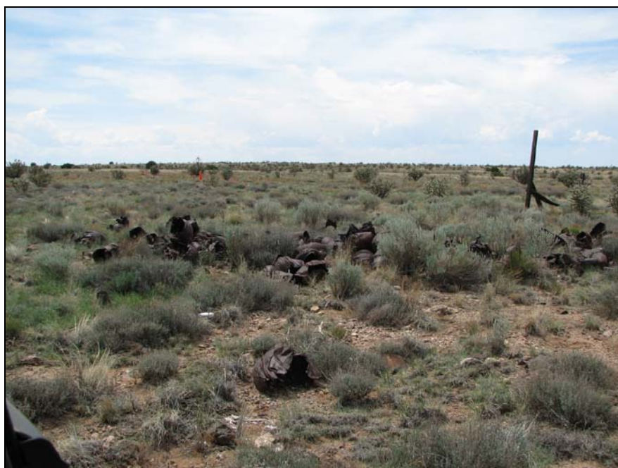
Figure 5. Photograph, looking north across the center of the PBR S-12 target. The pile of M38 scrap in the center of the photograph was not detected by the airborne magnetometer survey.
