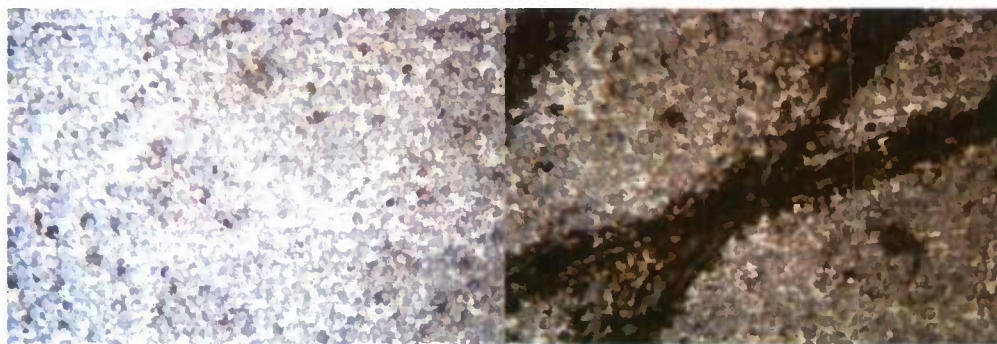
Figure 6: Mil-P resin with 10% microcapsules, before (left) and after (right) scratch.
