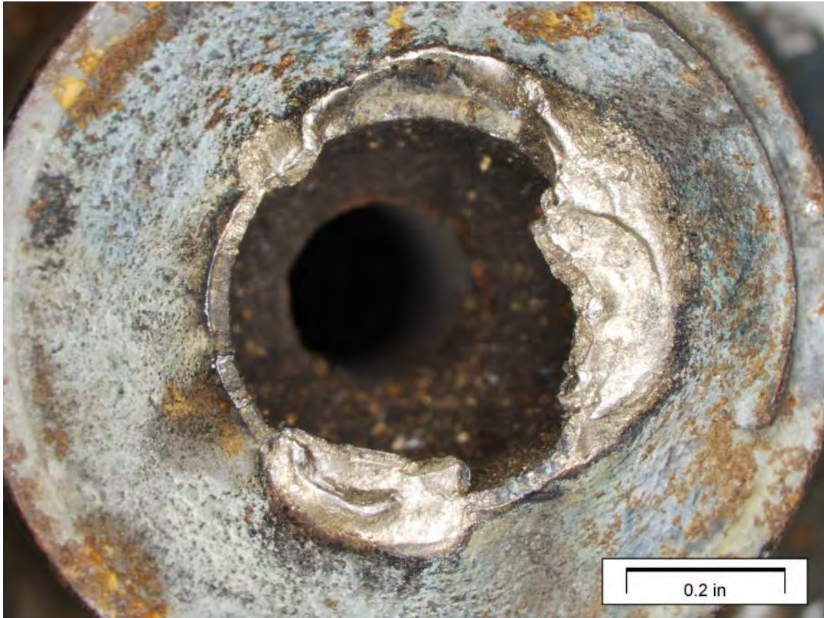
Figure 28. Greater detail of the marred areas and radial crack from the interior.
