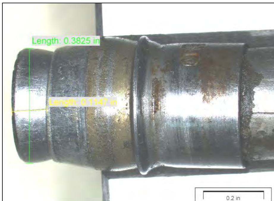
Figure 12. Intact end of the tube with measurements, side B.
