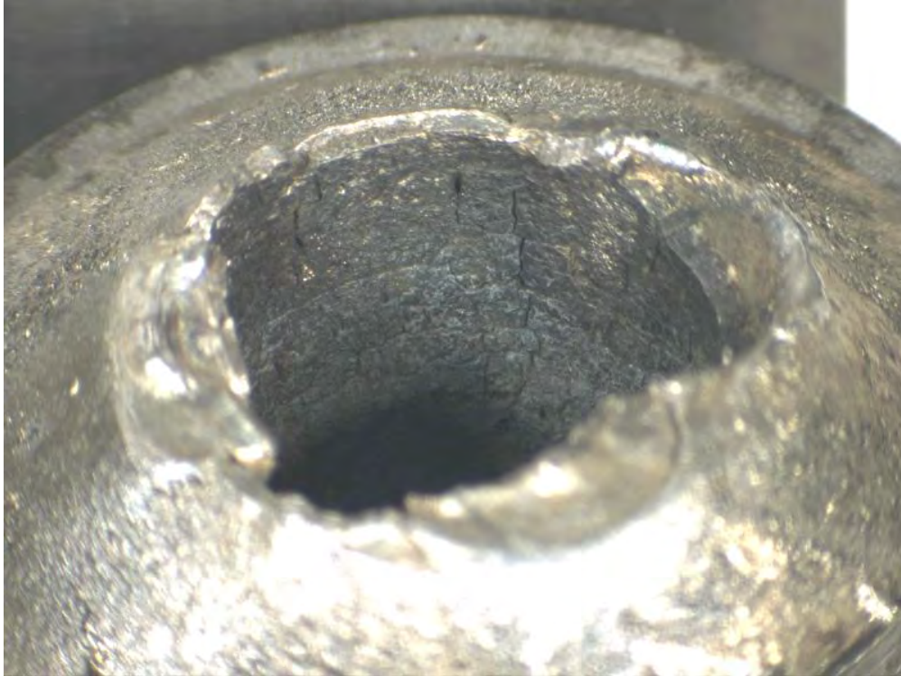
Figure 33. Interior cracked bore in figure 32 plus a 90° rotation.
