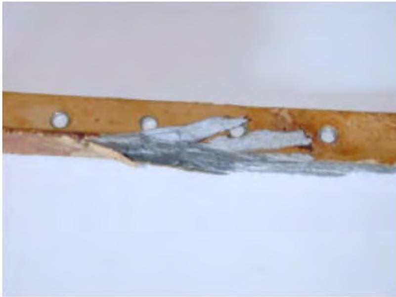
Figure 4-4: Exfoliation on a Breguet Atlantic Br. 1150 AA2024 Spar.
