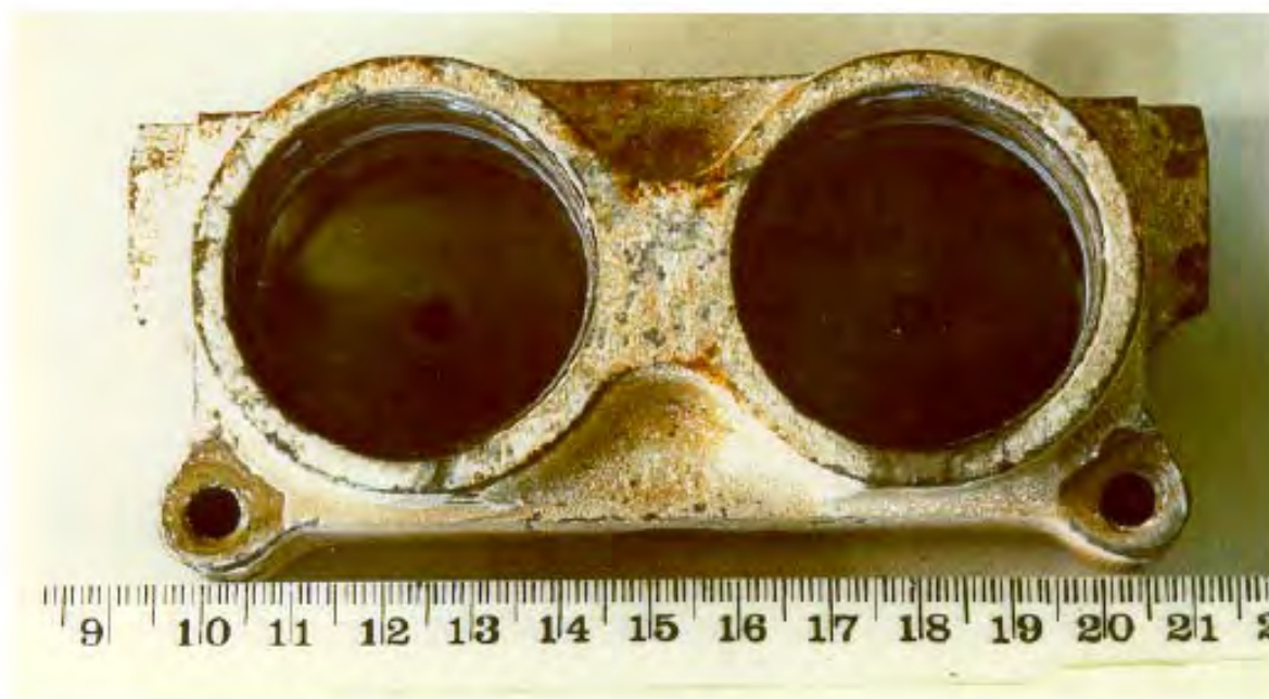
Figure 4-1: Uniform Corrosion on a Cadmium-Plated AM-X Air Combustion Chamber.
