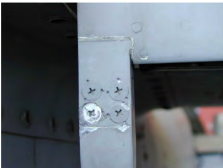
Figure 4-10: Galvanic Corrosion on the MB-339 between Mg Alloy Trim and Aluminum Rivets.
