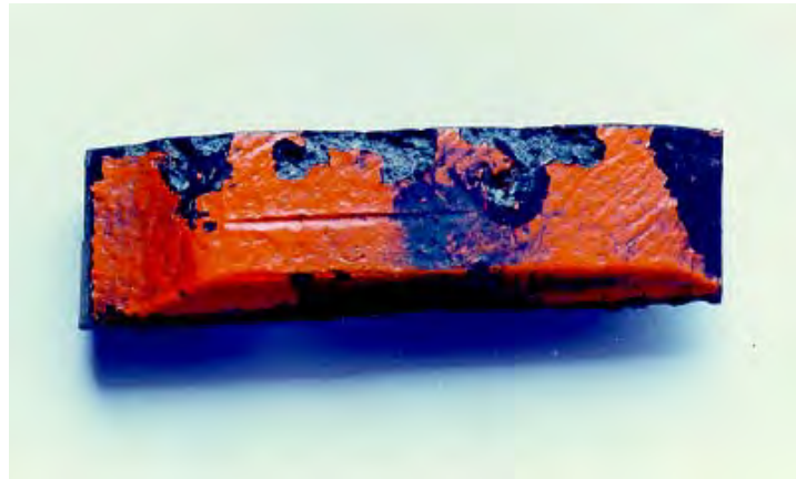
Figure 4-7: Pitting Corrosion on MB-326 Balance Tabs.
