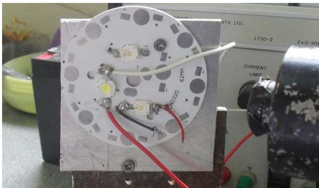
Figure 19. 1W OSRAM LED on Aluminum Substrate using CNTs/In composite as the thermal layer
