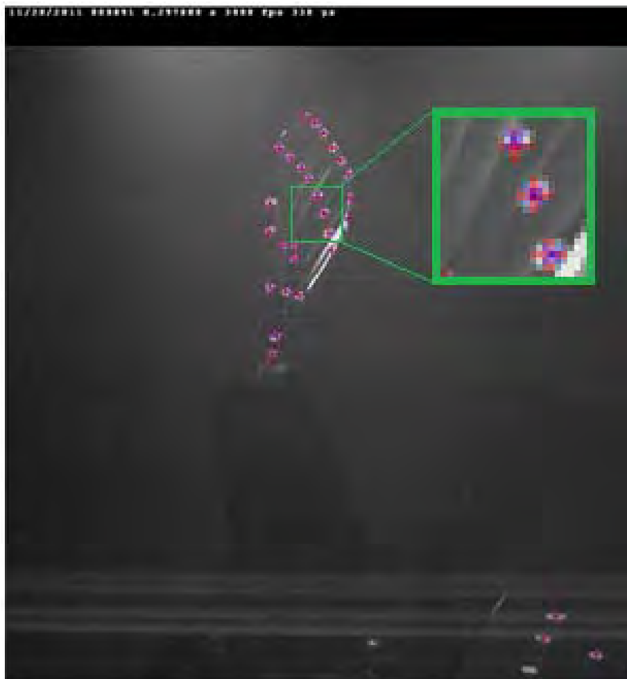
Figure 34: Top of the leading edge stroke with pixel and subpixel markings.
