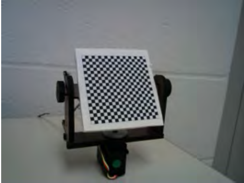
Figure 10: Pan-tilt calibration tool with calibration grid.
