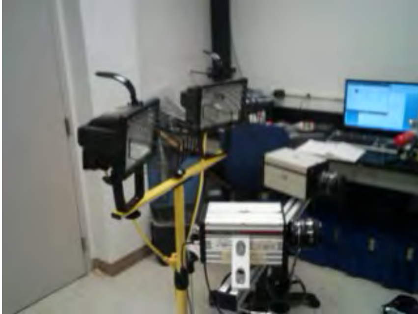
Figure 9: Cameras on common mount with halogen lamps.
