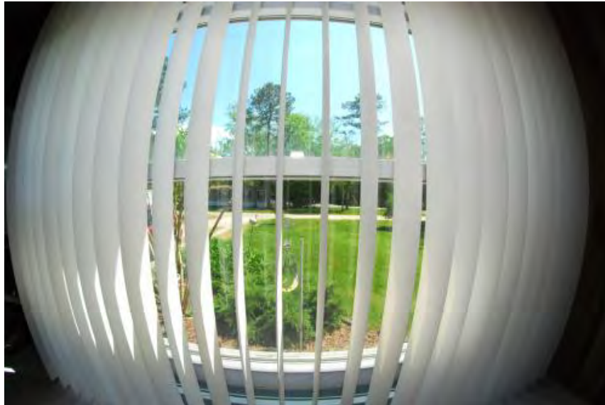
Figure 4: Vertical blinds photographed with a fisheye lens to show radial distortion.
