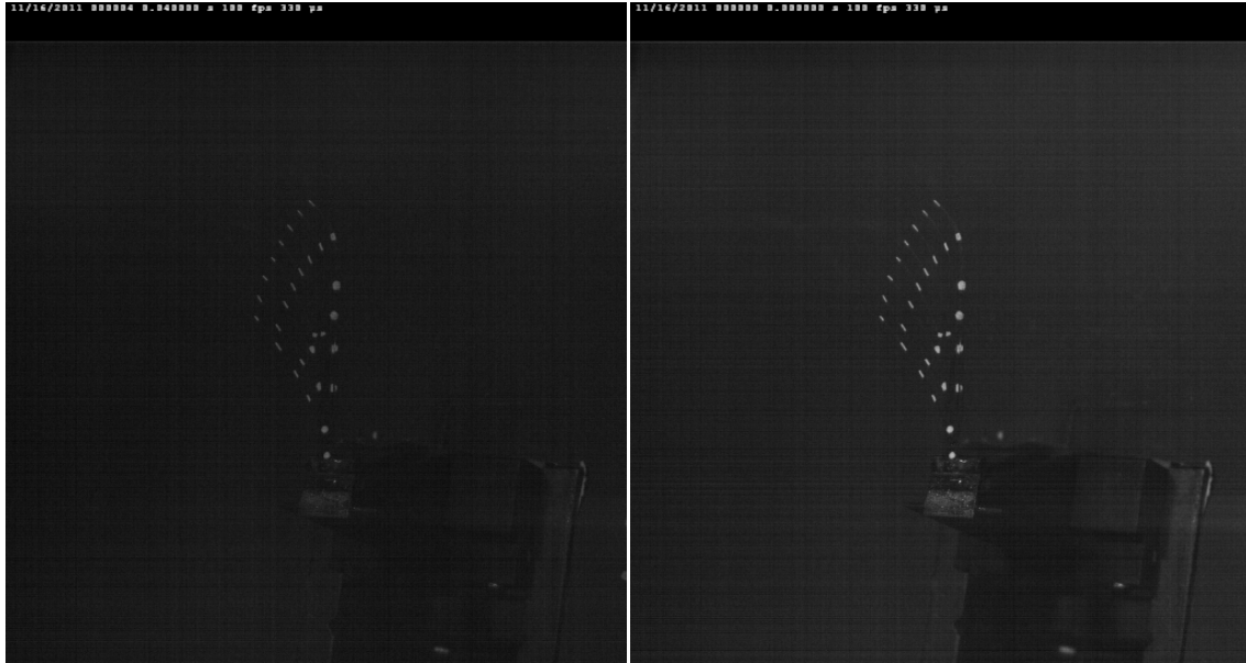
Figure 8: Left f/5.6, right f/4, note increased light and point visibility.
