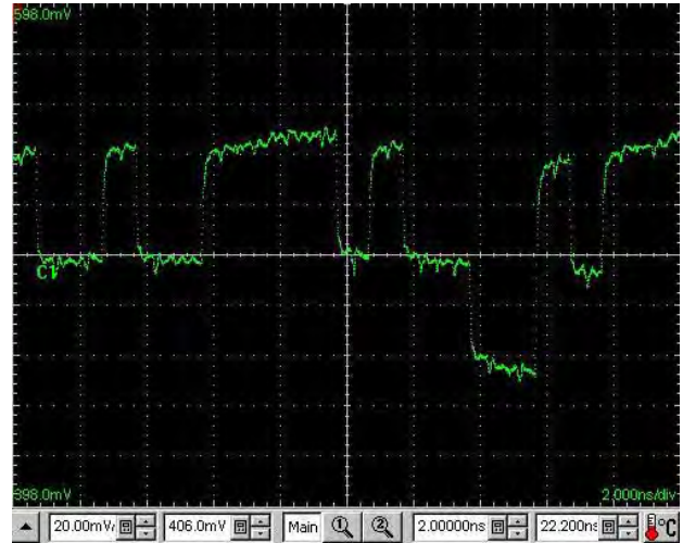
Figure 64 Random data stream showing taps 1 & 2 off and the final remaining tap on
