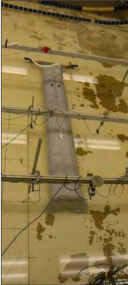
Figure D - 7: 0° breakwater configuration
