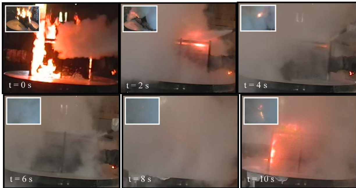
Figure 15. Sequence Showing Extinguishment Using PKP and Reignition at 7.5 s
