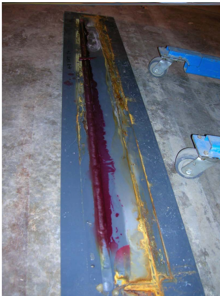
Figure 14.24: Penetration of dyed TCE into the silicone seals of SB 1-2.
