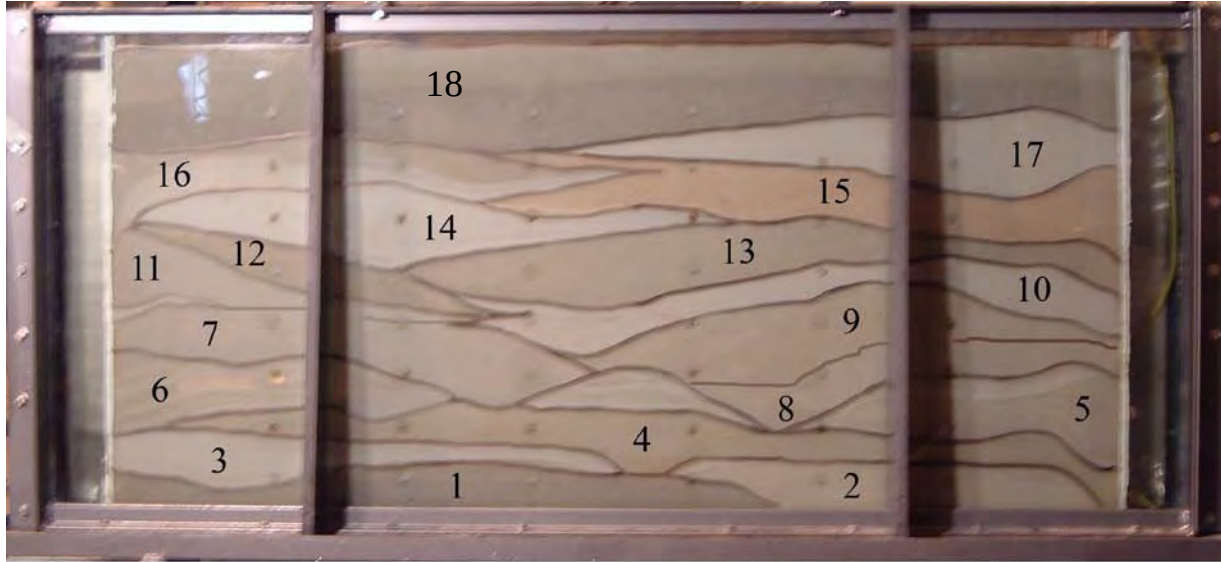
Figure 13.2: Photograph of synthetic heterogeneous aquifer created via cyclic flux of sediment-laden water [after Illman et al. , 2010].
