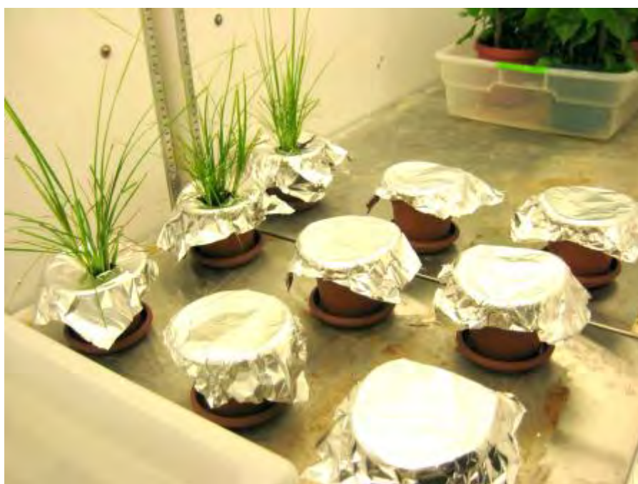
Figure 37. The experimental setup for the RDX microcosm study. Includes three replicates planted in soil from Eglin AFB with Bahiagrass Pensacola, three with excised Bahiagrass Pensacola roots, and three unplanted. All replicates were covered with aluminum foil to prevent the growth of phototrophic organisms. Not shown: the poplar and excised poplar root microcosms.
