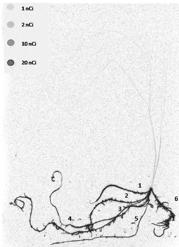
Figure 25. Phosphor imager autoradiograph of switchgrass 48 h after exposure to [U- 14 C]-TNT. The upper left corner shows the aliquots of [U- 14 C]-TNT of known radioactivity used as calibrators to calculate distribution of radioactivity in the plant. Numbered roots correspond to values given in Table 5.
