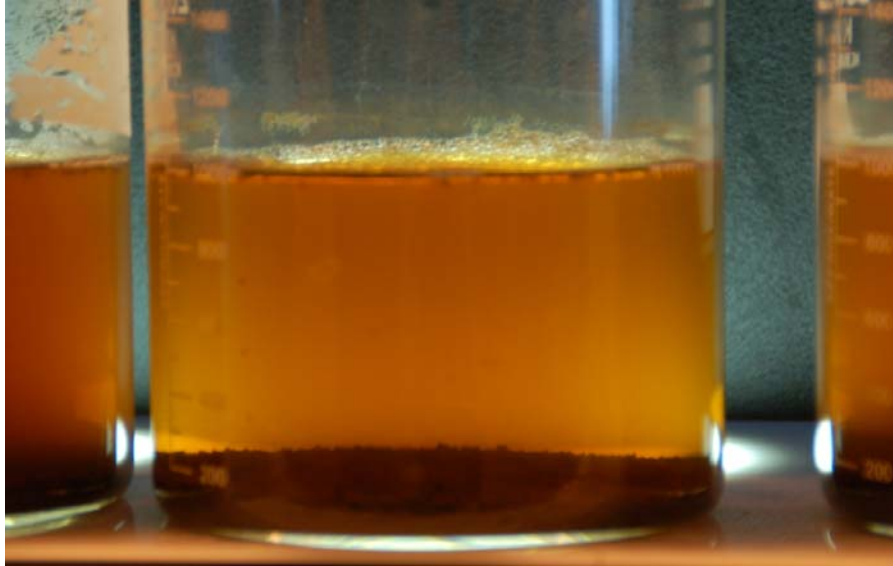
Figure 6-15. Separated solids in Run 5 coagulation/flocculation testing.
