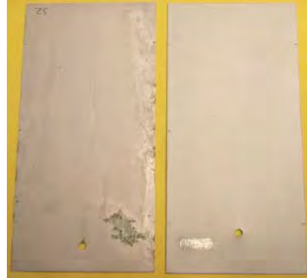
Figure 5-52 Back side of sample S2 from S series after 2205 hours salt fog testing (left panel), Non-salt fog tested zeolite panel with small area of zeolite removed, exposing bare metal (right panel).
