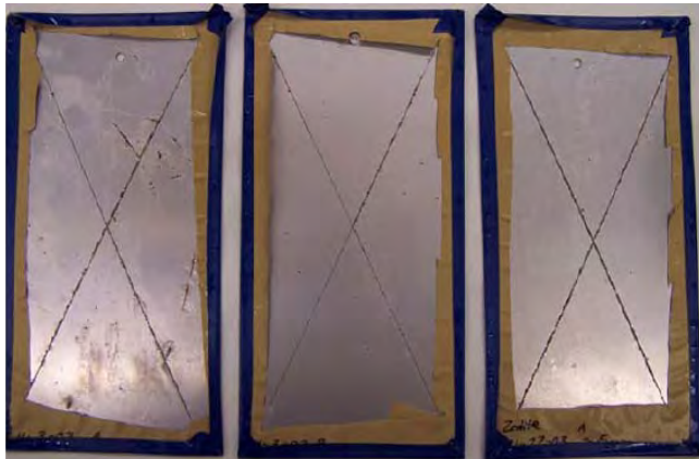
Figure 5-67 Exposed zeolite surface after 524 hours of exposure after CARC removal.
