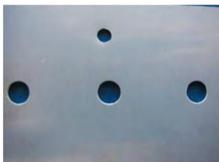
Figure 5-30 Photograph of a ZSM-5 coated AA-2024-T3 panel with punched holes
