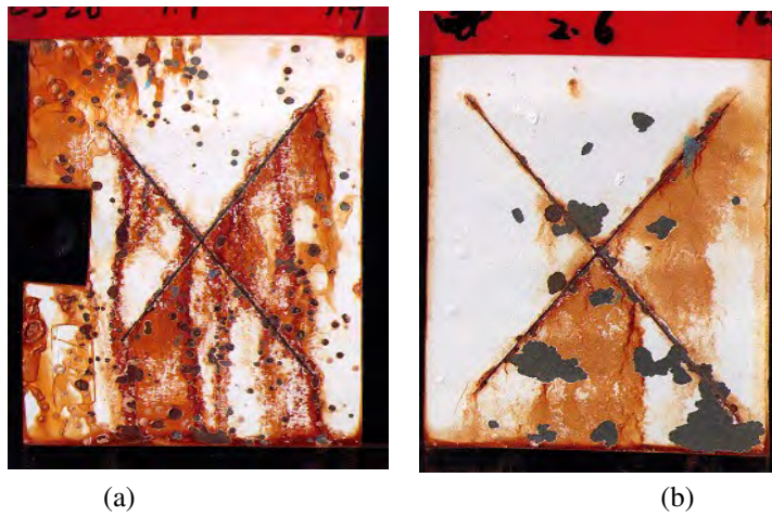
Figure 6. CRS with MIL-P-53030C after 500 hrs of SST; (a) ECO-008, (b) DoD-P-15328D.
