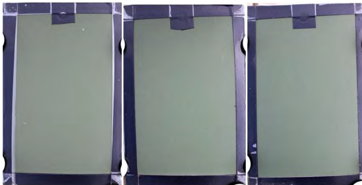
Figure 40. CRS panels coated with ECO-008/MIL-DTL-53022D/MIL-DTL-64159A after 6 months
