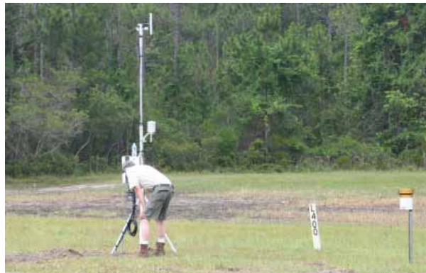
e. weather station with windset and rain gage (mounted on post, right side of photo)
