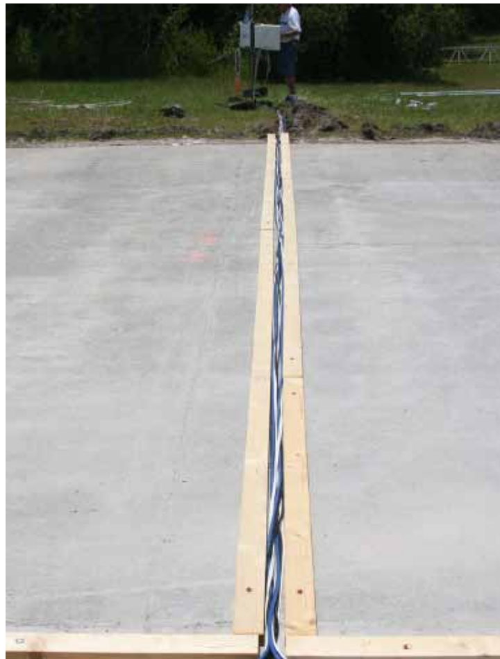
Figure 13. Photograph showing protected instrumentation wires routed to data acquisition system off the runway edge.
