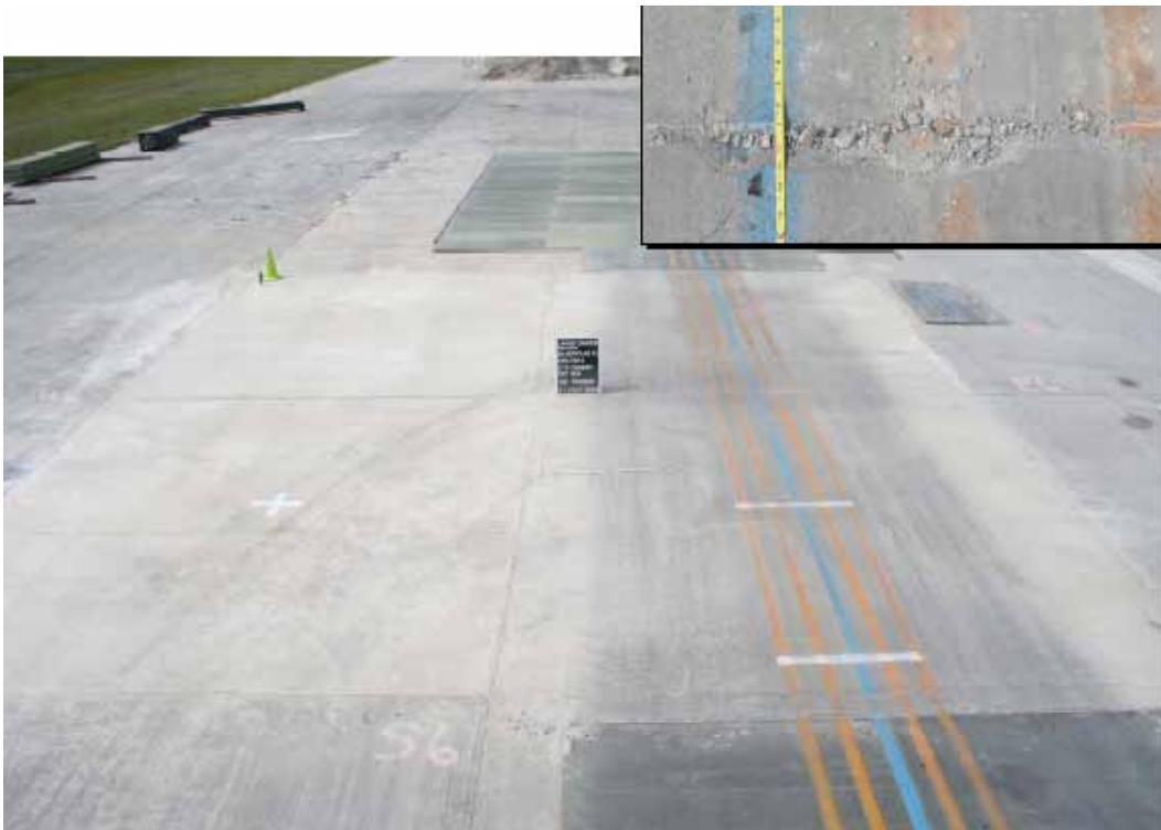
Figure 145. Crater 6 after 528 completed load cart passes.
