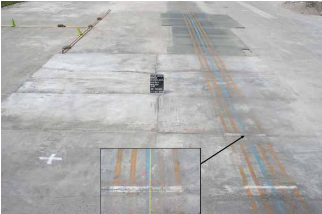
Figure 144. Crater 5 after 528 completed load cart passes.
