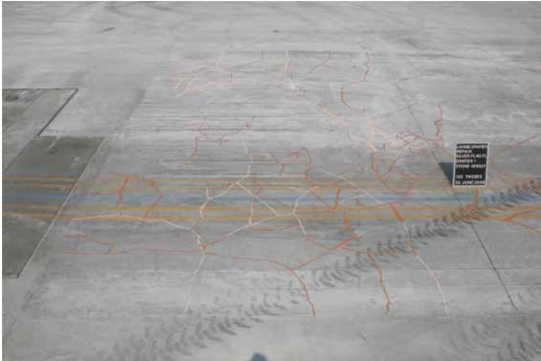
Figure 135. Crater 1, Stone & grout after 102 passes of load cart.
