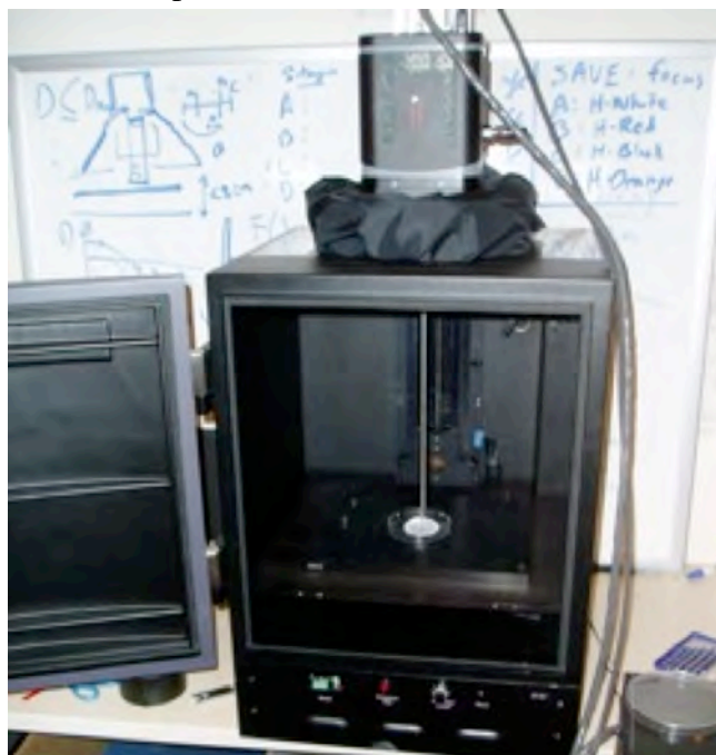
Figure 1: Small-animal imaging box fabricated to provide proof-of-concept and aid in technique and nanoparticle development.
