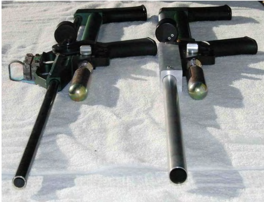
Figure 7: The 13mm Dan-Inject rifle on the left and the modified rifle with the 20mm barrel on the right.
